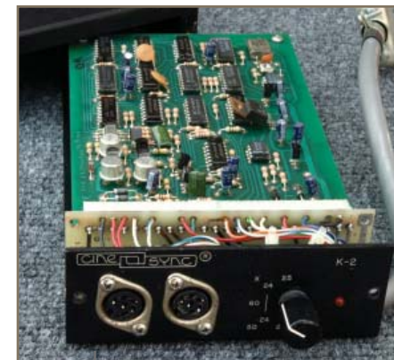
A Cine-Sync K-2 to link KEM editing machines. Denecke made and sold about 400 of these boxes.
